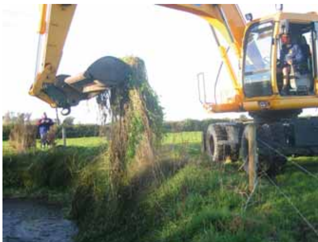
A weed cleaning rake bucket minimises damage.
